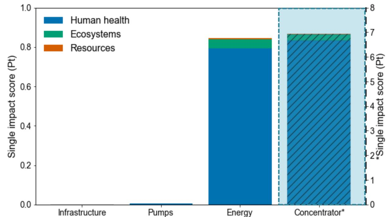
**Concentrator equipment has the highest impact in the system**
